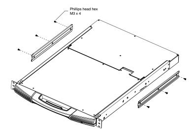
Packing material has been inserted to protect the KL9108 / KL9116 during shipping. Slide the LCD module out until the packing material is visible. Remove the packing material before installing the unit, as shown in the diagram below.
